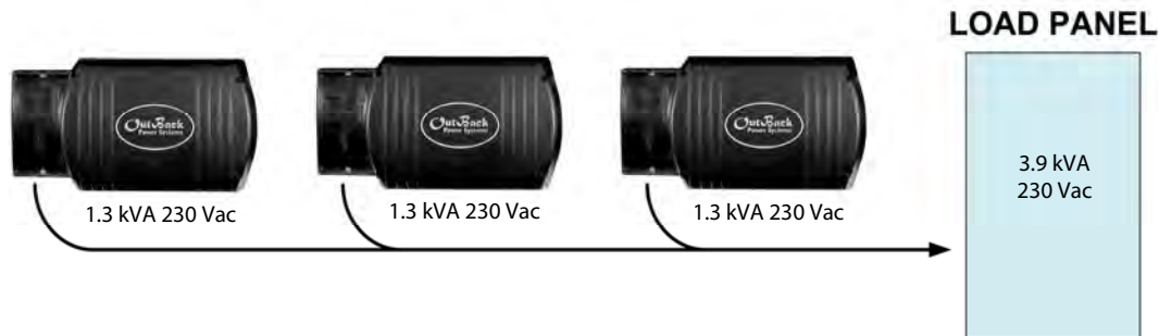
Figure 20 Example of Parallel Stacking Arrangement (Three Inverters)
