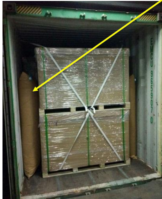
S11: Stack pallets in container and fix the outermost row with straps and gasbags in case of left or right slipping.
