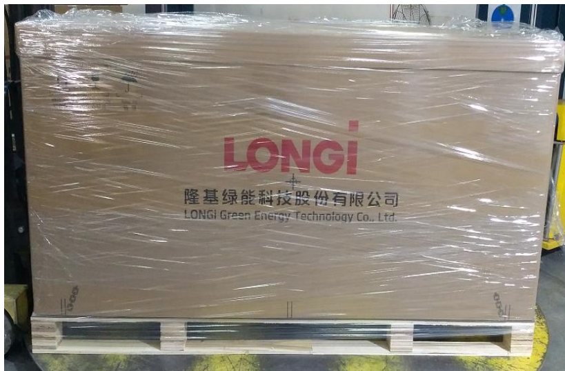
S9: Cover the package cap and wrap the paper package with waterproof film;
